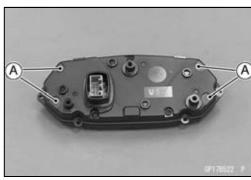
Remove: Screws [A] Lower Meter Cover [B]
