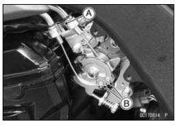
◆ Loosen the throttle body assy holder clamp bolts [A].
