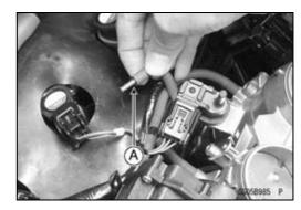
Connect a vacuum gauge (special tool) and hoses [A] to the fittings on the throttle body.
