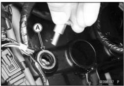
• Tighten the cover bolts following the specified tightening sequence.
