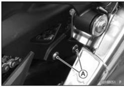
Remove: Quick Rivets [A] Mud Guard [B]
