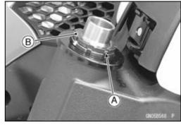
Pushing up the stem base, and remove the steering stem nut [A] with stem cap [B].
