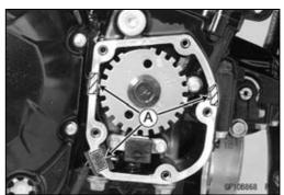
Replace the O-ring [A] in the crankshaft sensor cover with a new one.
