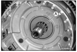
• Install the washer [A] so that the "OUTSIDE" mark [B] faces outward.
