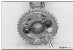
Install the camshaft sprockets so that position the timing marks [A] outside (Engine Number:ZRT00DE016593 ~)
