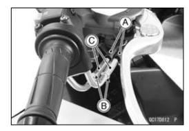
Remove: Bolts [A] Throttle Pulley Cover [B]
