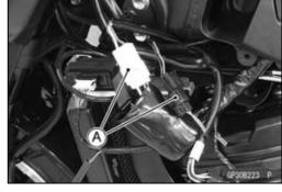
Remove: Bolts [A] Ignition Switch Cover [B]
