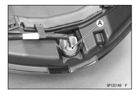
• Pull out the bulb [A] straight from the socket.
