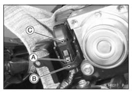
Remove: Bolts [A] ABS Hydraulic Unit [B]
